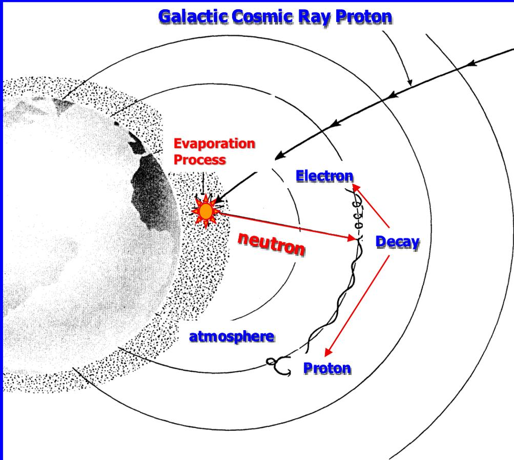
CRAND electrons are mostly from the  $\beta$ -decay of thermal neutrons:
