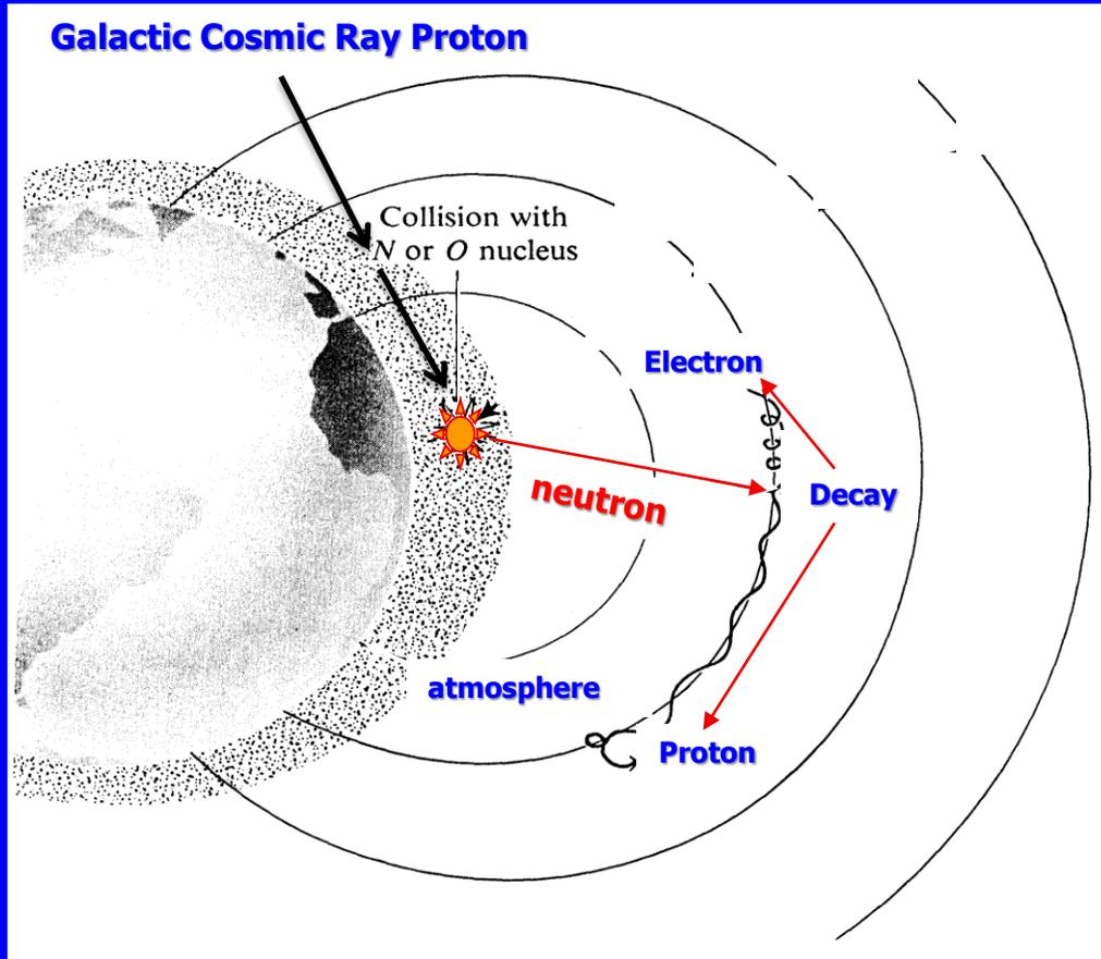
Fast neutrons made by direct interaction of high-energy cosmic rays: knock-on neutrons
