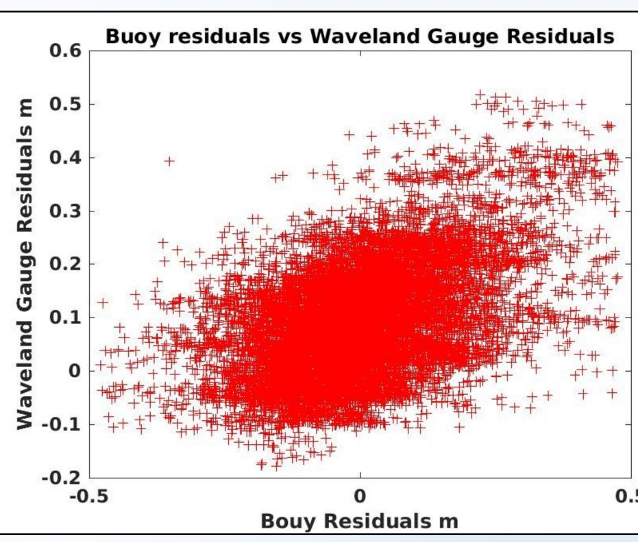
Figure 5: Plot of buoy and Waveland gauge tidal residuals
