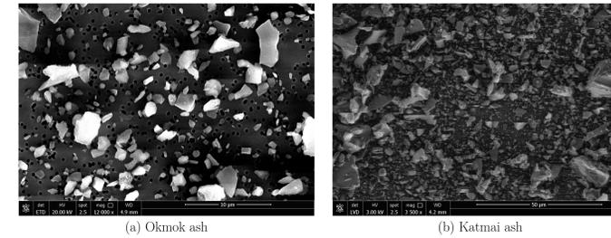
Figure 4: Scanning Electron Image of volcanic ash particles collected on a nuclepore filter
