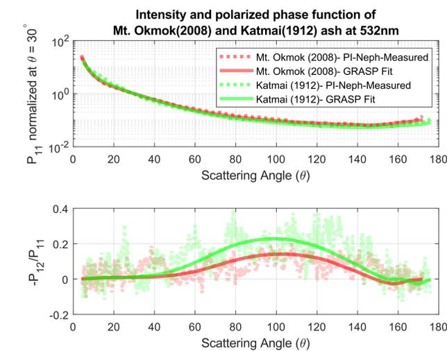
Figure 5: P<sub>11</sub> and -P<sub>12</sub>/P<sub>11</sub> of volcanic ash samples measured using PI-Neph
