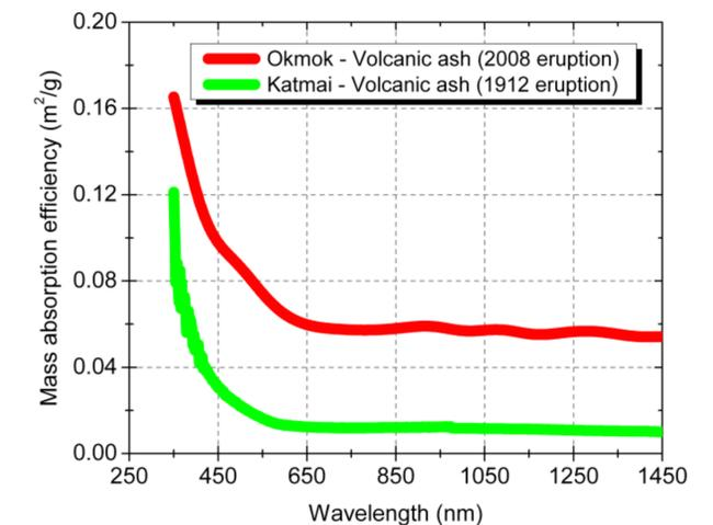
Figure 7: Mass absorption efficiency  $\alpha_{abs}$  of the volcanic ash samples measured using a reflectance measurement setup mentioned in technique described by Rocha-lima et. al 2014[5]
