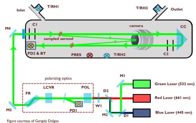
Figure 3: Polarized-Imaging Nephelometer (PI-Neph)
