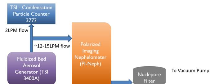
Figure 2: Schematic diagram of the experimental setup
